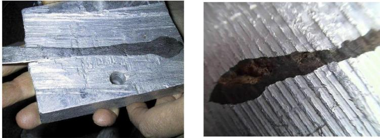
How did John get liquid aluminium to work this way? We can see on the right hand side the knife is quite well embedded into the metal block, though over to the left it does not seem fully fused. The marks of the surface of the block go in different directions, and certainly do not look like the results from using a grinder. In the picture on the right, why would molten aluminium would have left the wood unburned?
